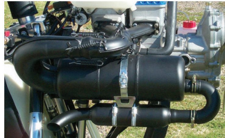
PHOTO OF INSTALLED EXHAUST WITH AFTER SILENCER.
