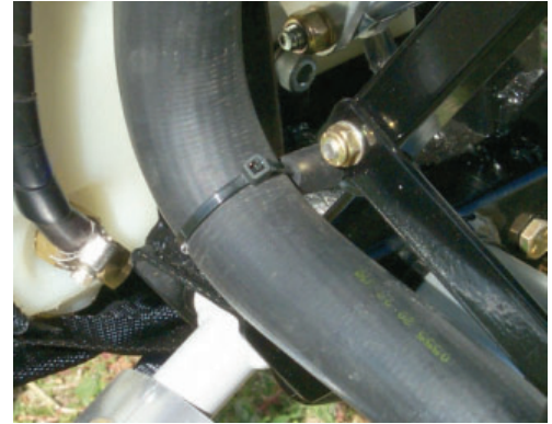
PHOTOS SHOW CABLE TIED FUEL HOSE SPACERS.
