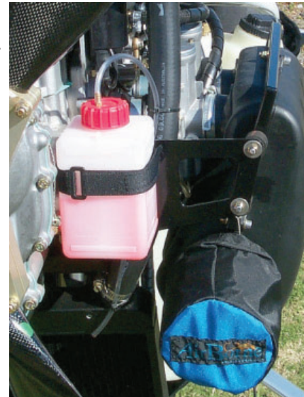
PHOTO SHOWS GAP BETWEEN RADIATOR AND AIR FILTER
