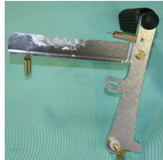
PHOTO SHOWS SPRINGS AND DRI LUBE INSTALLED CORRECTLY.
