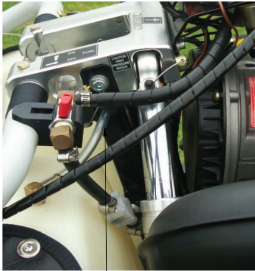
PHOTO 1. FUEL TAP WITH HOSES
