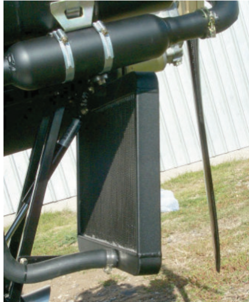
PHOTO SHOWS INSTALLED RADIATOR.
